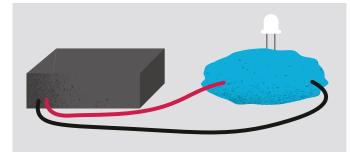
Now separate the conductive dough into two pieces. Make sure the two pieces are not touching. Plug one wire from the battery pack into each piece of wire. Bridge the gap with an LED. Does the LED light up now?
